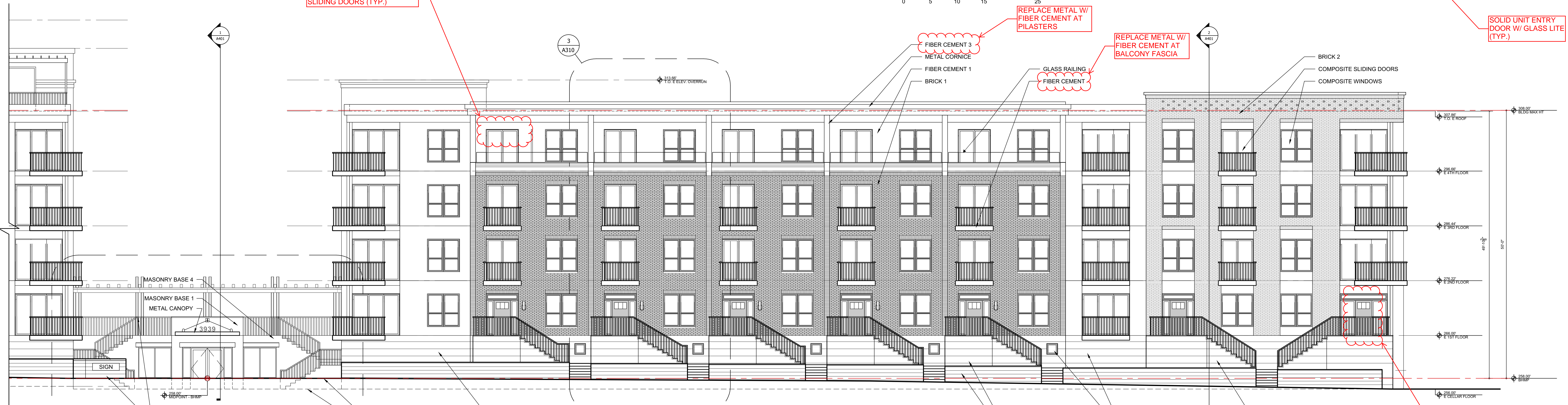
2 EAST BUILDING - SOUTH ELEVATION SCALE: 1/8" = 1'-0"
