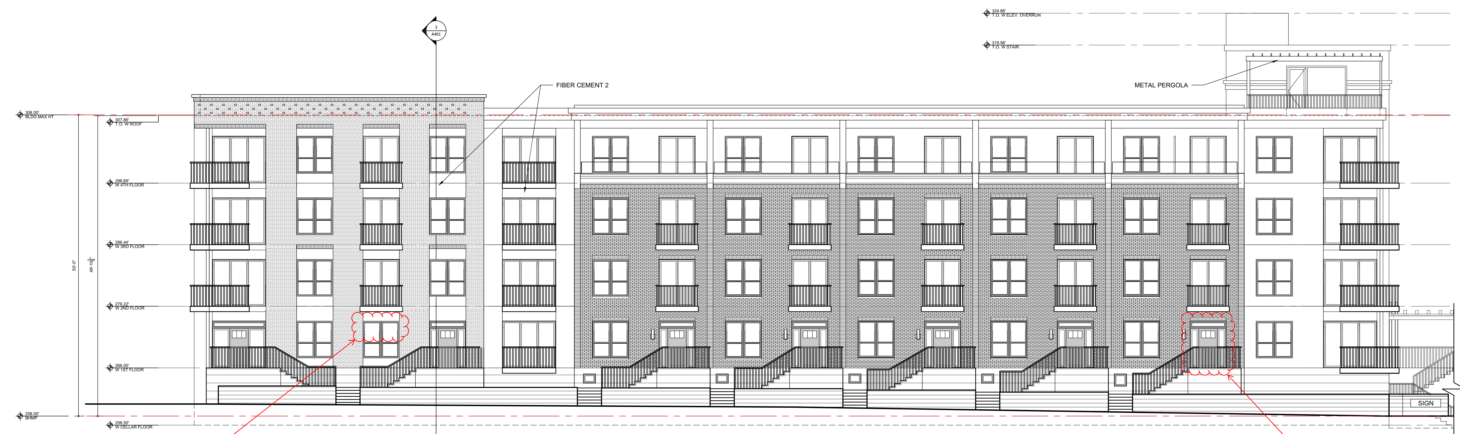
3 WEST BUILDING - SOUTH ELEVATION SCALE: 1/8" = 1'-0"
