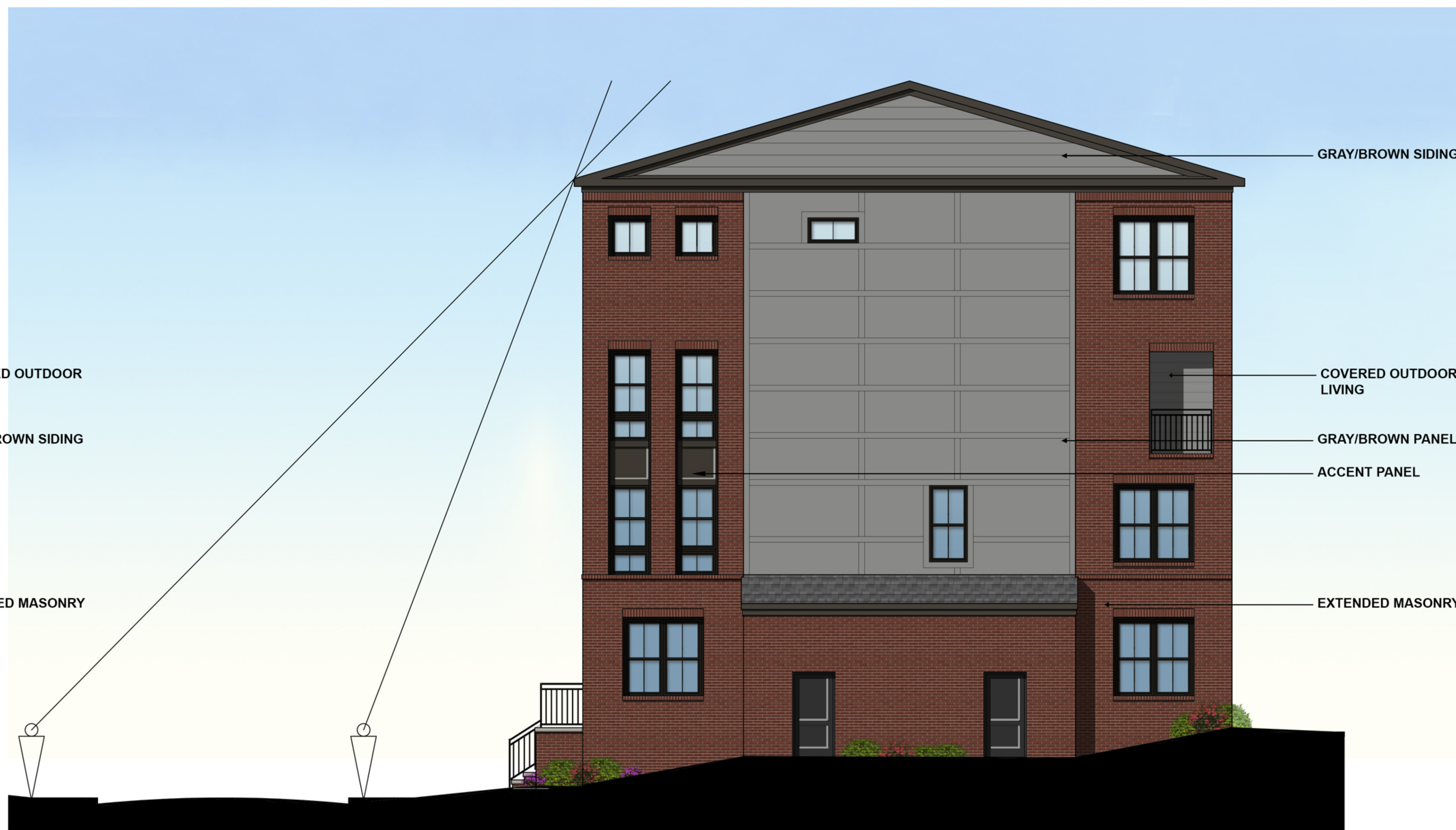
TYPICAL HIGH VISIBILITY END UNIT SIDE ELEVATION - 2 OVER 2 SHOWN WITH LINE-OF-SIGHT EXHIBIT (N.T.S.)
