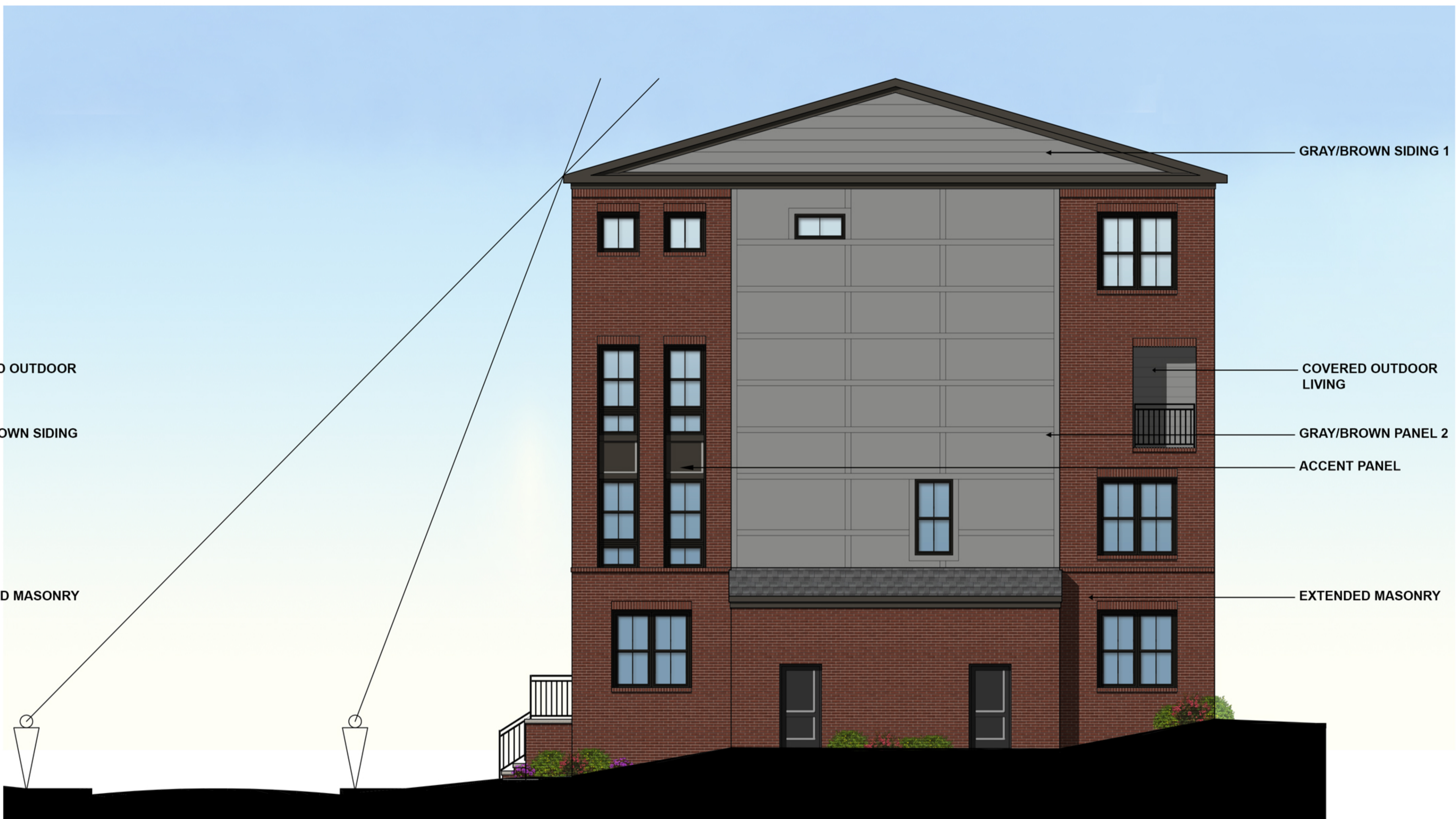
TYPICAL HIGH VISIBILITY END UNIT SIDE ELEVATION - 2 OVER 2 SHOWN WITH LINE-OF-SIGHT EXHIBIT (N.T.S.)
