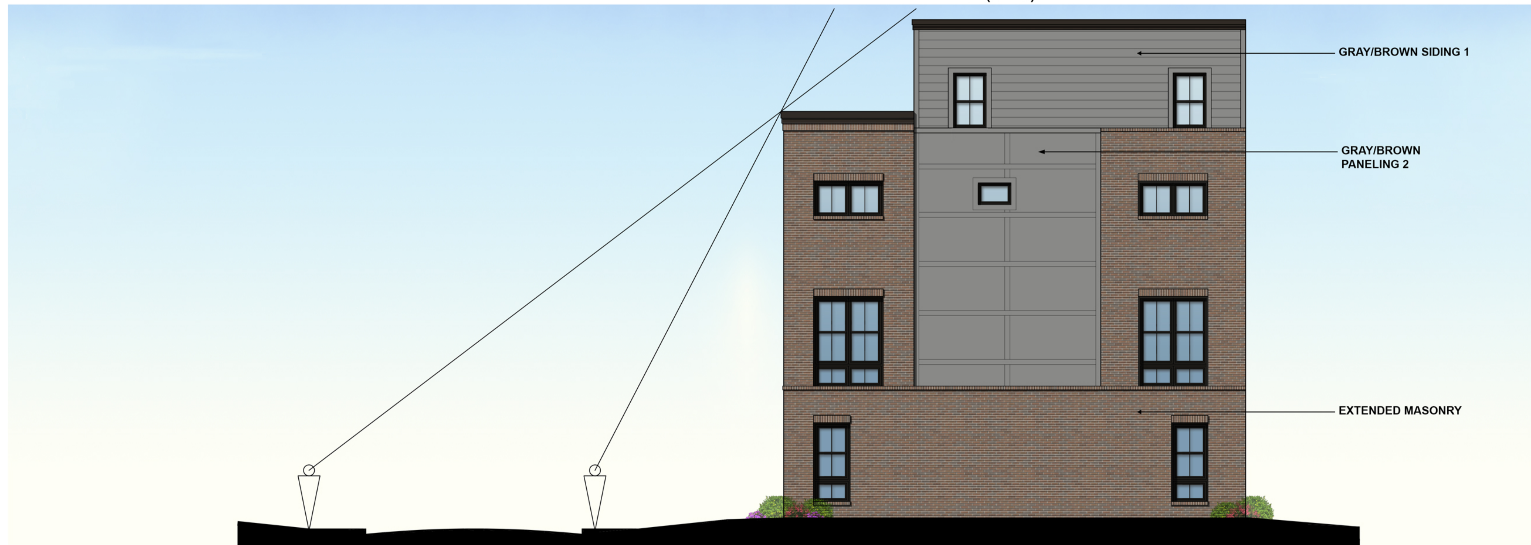
TYPICAL HIGH VISIBILITY END UNIT SIDE ELEVATION - 16' SHOWN WITH LINE-OF-SIGHT EXHIBIT (N.T.S.)
