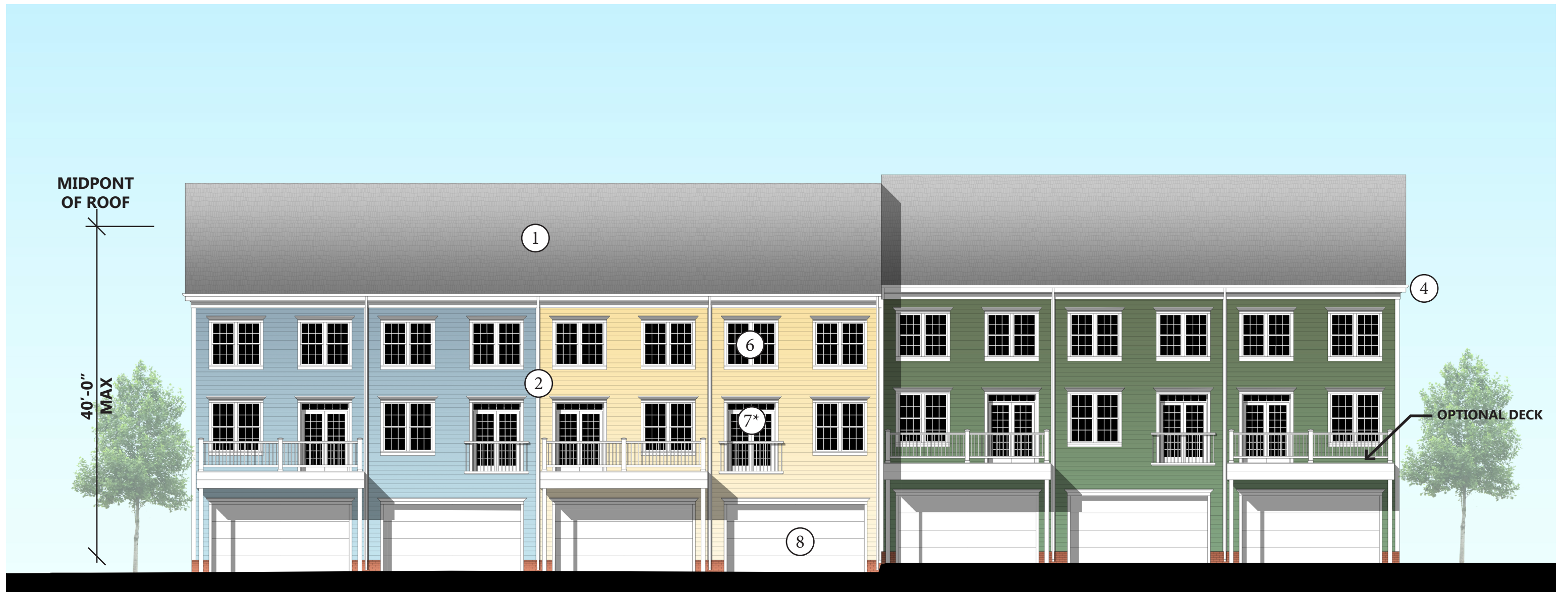
20' REAR LOADED TOWNHOUSES REAR ELEVATION
